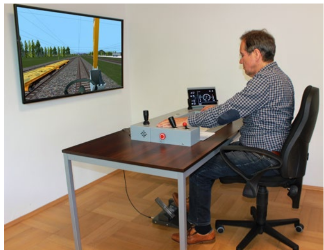
Familiar handling: control panel, pedal set, and joysticks Vertrautes Handling: Bedienpult, Pedalsatz und Joysticks
