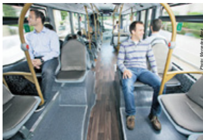
View of the passenger compartment: The extruded aluminium horizontal grab rails have an oval cross-section and a larger diameter, designed to make them especially easy to grasp. In addition, the new shape enables light fittings to be integrated in the grab rails, as well as exchangeable advertising inserts with clamp fastening, or even ticker-style displays in the grab rails – a completely new form of advertising.
