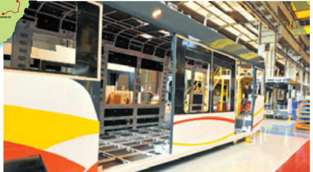
Vossloh Rail Vehicles, based in Albuixech near Valencia, Spain is responsible for the design, manufacture – the photo shows car bodies being assembled – and delivery of the new train-trams.
