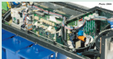
A look inside the SMA battery chargers for the "Civity" platform. Photo: SMA
