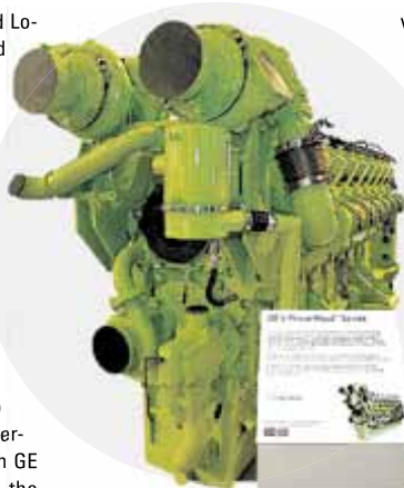
GE Transportation presented its new 16-cylinder diesel PowerHaul locomotive engine.
