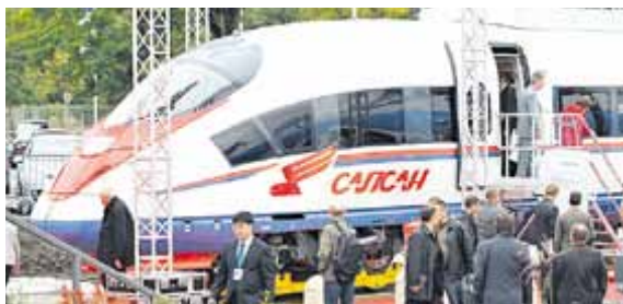
The Velaro RUS had to be brought to Berlin on a special undercarriage owing to its broad-gauge configuration. Photo: Messe Berlin
