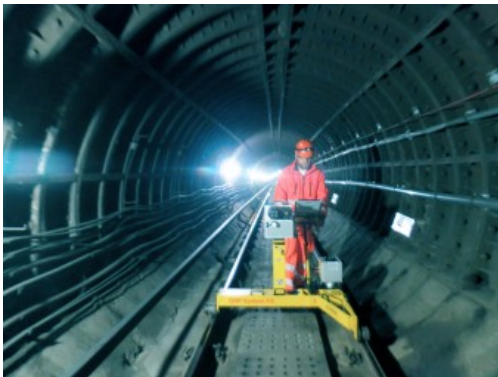
Conducting measurements with the Amberg IMS 5000
