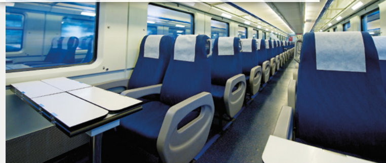
Seats made from fire-retardant foams
