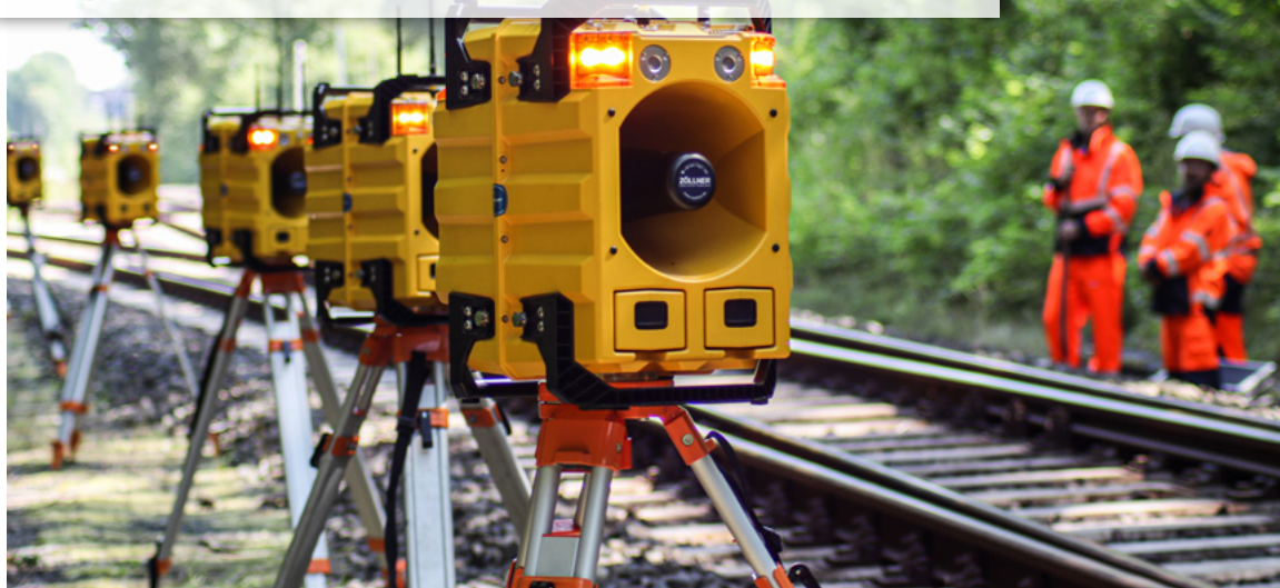
The automatic light and sound warning system warns of an approaching train
